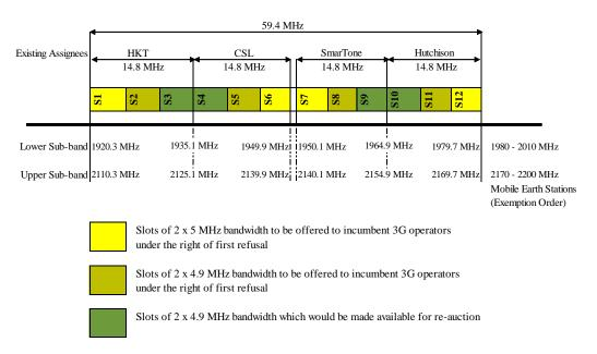
Figure 2 - Proposed Band Plan for Re-assignment of the Frequency Spectrum in the 1.9 - 2.2 GHz Band
